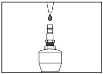
Figure 1. Lubricating nailer via air inlet.
